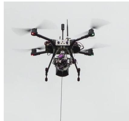
For the Indoor Positioning System, Delft Dynamics has tested a couple of SLAM-Sensors such as a tracking cam and a Lidar laser system. The tracking cam can provide data fast enough to use it for stable control of the mobile platform. Delft Dynamics has made preliminary design concepts for the Sensor Placement System for the wall thickness measurements. These concepts will be further developed in the coming period.
