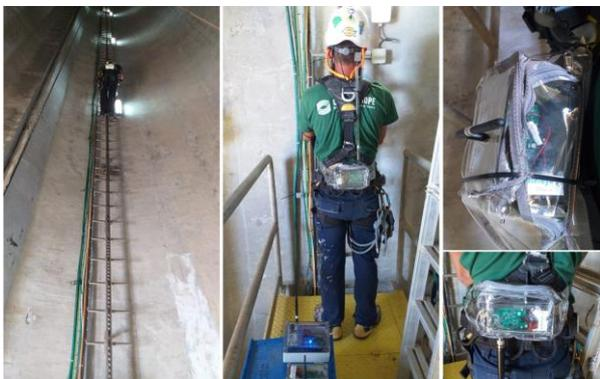
Figure 6. Test setup inside the wind turbine tower
