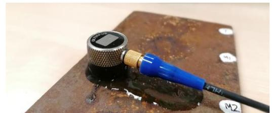
Figure 1. Test setup for ultrasound sensor nodes
