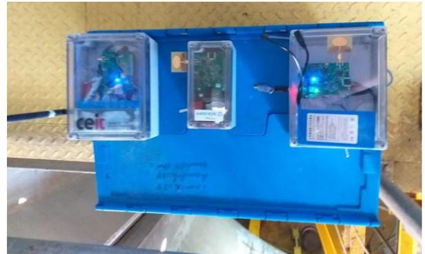
Figure 7. Fixed nodes located on the access platform
