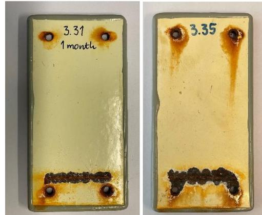
Figure 3. Corrosion creep on 1-month sample (left) and on 5-months sample (right)
