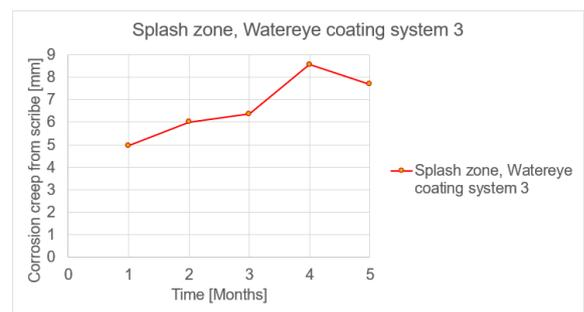
Figure 4. Corrosion creep from scribe
